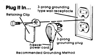
A 115 Volt, 60 Hz., AC only, 15 or 20 ampere fused electrical supply is required. It is recommended that a separate circuit serving only this appliance be provided. The receptacle should not be controlled by a wall switch or pull chain.
